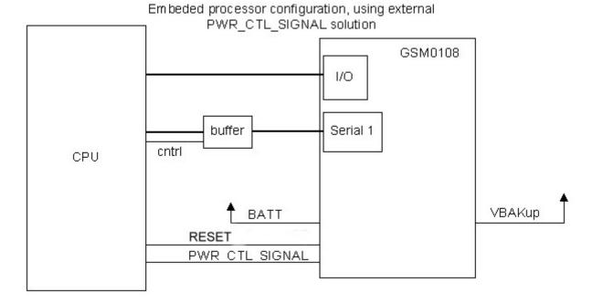
Figure 11 Power Control Signal (using external processor)
